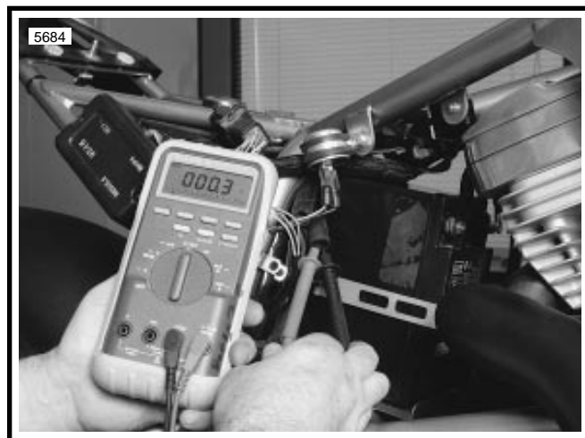
Figure 7-24. Check for Stator Resistance
