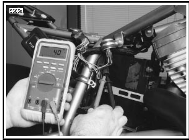
Figure 7-25. Check Stator AC Voltage Output
