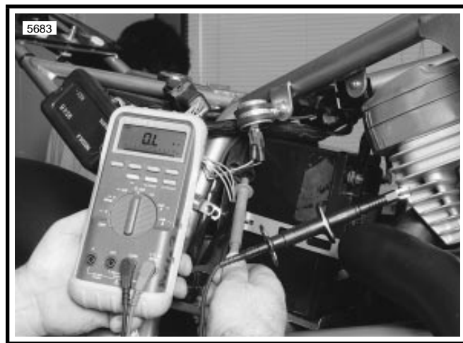
Figure 7-23. Test for Grounded Stator
